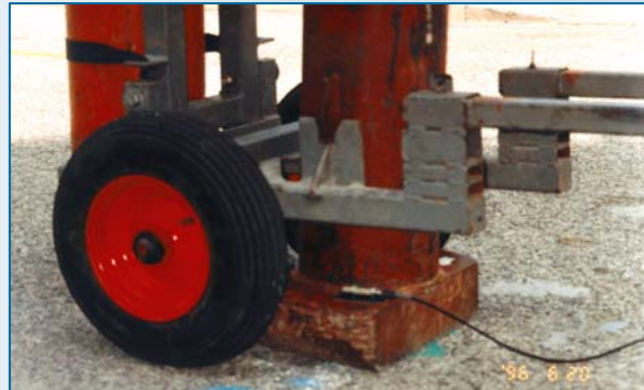
SEISMOGRAPH TRIGGER ATTACHED TO BASE PLATE
