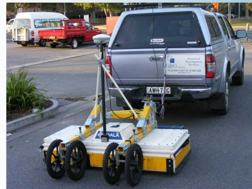
Figure 1: MIRA 3D system behind the GBG survey vehicle.
