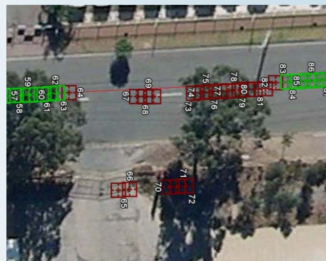
Figure 4 : Post-process of GPS data of each GPR profile. GPS positions with high error (in red) will be removed from profile path. Positional accuracy can be achieved to less than ±5 m every 1 km.
