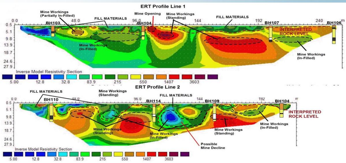
**Mapping of filled open cast coal mine workings** – The resistivity profile below was recorded in a region in Cumbria United Kingdom which was known to have been part of an open cast mine in the 1970's and was subsequently filled and returned to farming land. The purpose of the survey was to map the extent and depths of the mine pits to help establish the bearing capacity of the ground before the proposed construction of a wind farm.
