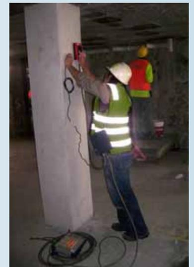
1.5GHz ANTENNA USED TO SCAN CONCRETE COLUMNS
