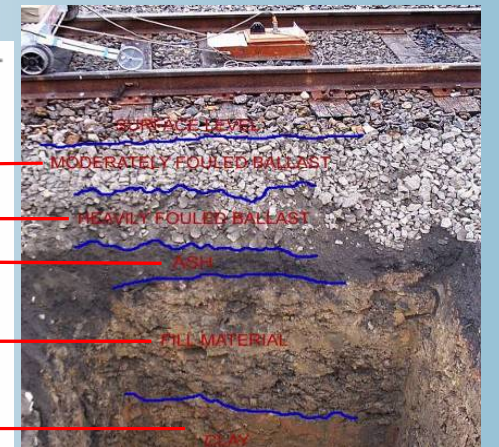
Test pit used as a calibration during the investigation.
