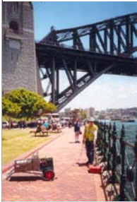
GROUND PENETRATING RADAR SURVEY USING 500MHz ANTENNA
