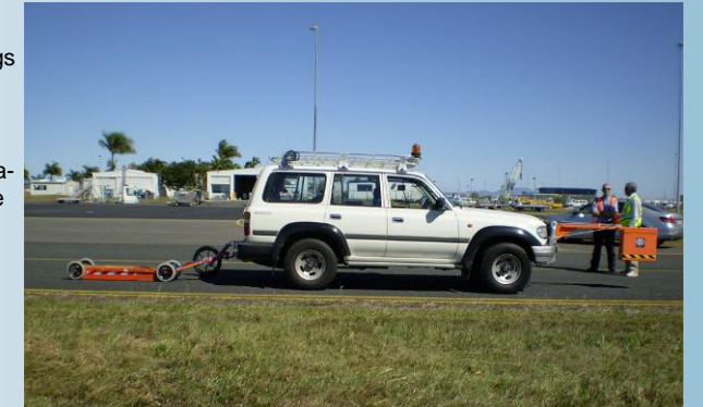
4WD with GPR system, ground coupled antennae are towed in the trolley behind, whilst the airhorn antenna is mounted at the front.
